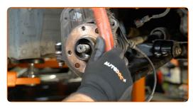
64 Install the brake disc.
