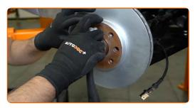
20 Remove the brake disc.
