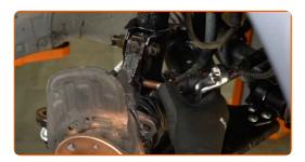
Unscrew the fastener connecting the ball joint to the steering knuckle. Use a combination spanner #16. Use a drive socket #16. Use a ratchet wrench.
