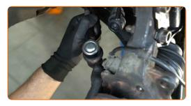
Tighten the fastening nut connecting the tie rod end to the steering knuckle. Use a drive socket #17. Use a torque wrench. Tighten it to 35 nm torque.
