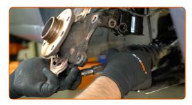
Remove the fastening bolt.
