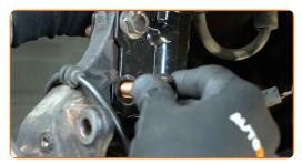
Screw in the fasteners connecting the suspension strut to the steering knuckle. Use a combination spanner #18. Use a drive socket #18. Use a ratchet wrench.
