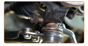
Screw the fasteners of the ball joint. Use a combination spanner #16. Use a drive socket #16. Use a ratchet wrench.
