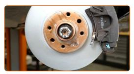
Treat the surface where the brake disc contacts the wheel rim. Use copper grease.
