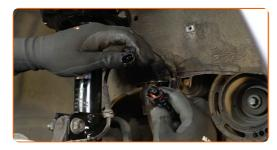
Disconnect the ABS sensor wiring.
