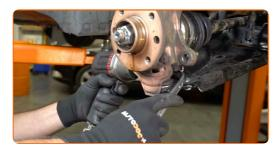
Remove the fastening bolt.
