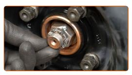
79 Treat the CV axle fastener. Use copper grease.
