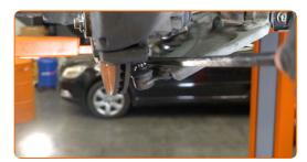
Remove the front fastener of the control arm. Use a drive socket #18. Use a ratchet wrench.
