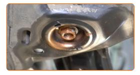
27 Treat the contacting surface. Use copper grease.
