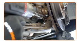
Remove the fastening bolt. Use a combination spanner #16.
