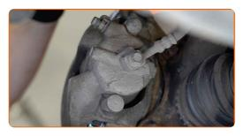
20 Install the brake caliper retaining spring.
