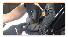
Unscrew the brake caliper fastening. Use HEX No.H7. Use a ratchet wrench.
