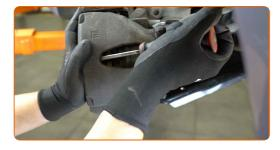
11 Remove the brake caliper.
