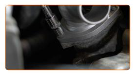
Tighten the thermostat housing fasteners. Use a drive socket #E8. Use a torque wrench. Tighten it to 7 nm torque.
