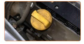
Unscrew the coolant reservoir cap.
