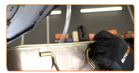
Open the coolant drain tap. Use a flat screwdriver.
