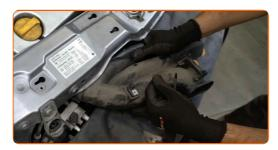
Unscrew the engine cover fastener. Use Torx T30. Use a ratchet wrench.
