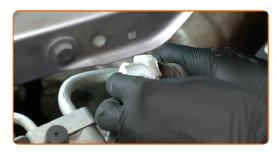
Unscrew the thermostat housing fasteners. Use a drive socket #E8. Use a ratchet wrench.
