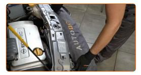
Unscrew the fasteners of the air distribution housing assembly. Use Torx T20.
