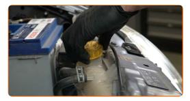
Pour coolant in the coolant reservoir.
