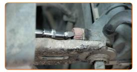
Drain the coolant from the engine.
