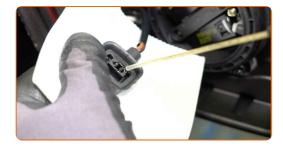
Attach the mirror heater connector.
