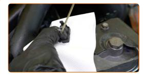
Plug in the connector of the coolant temperature sensor.
