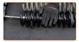
Replacement: coil springs – MERCEDES-BENZ W124 Estate (S124). Tip from AUTODOC:
