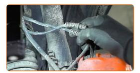
Unscrew the lower fasteners on the shock absorber. Use a drive socket #19. Use a ratchet wrench.
