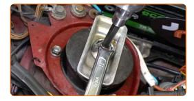
Replacement: suspension strut – MERCEDES-BENZ W124 Estate (S124). Tip:
