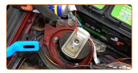
Loosen the fasteners of the upper strut mount. Use a drive socket #13. Use a ratchet wrench.
