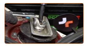
Unscrew the fasteners of the upper strut mount. Use a drive socket #13. Use a ratchet wrench.
