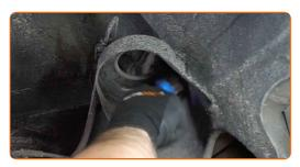
Clean the shock absorber mounting seats. Use a wire brush. Use all-purpose cleaning spray.
