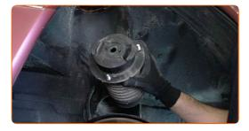
Remove the shock absorber dust boot and bump stop.
