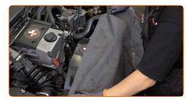
Release the air filter cover clips.
