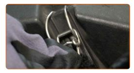
Remove the fender protection cover.
