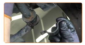
10 Remove the anti-roll bar.
