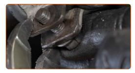
Tighten the fasteners on the anti-roll bar bush brackets. Use a combination spanner #13. Use a drive socket #13. Use a torque wrench. Tighten it to 20 Nm torque.
