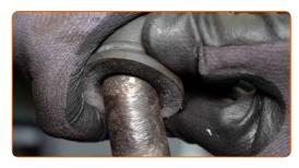
Clean the brackets of the anti-roll bar bushes. Use a wire brush. Use all-purpose cleaning spray.
