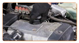
Unscrew the filter housing cap together with the old filter element. Use the 62-23F socket. Use a ratchet wrench.
