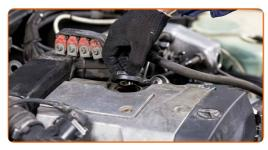
Tighten the oil filler cap.
