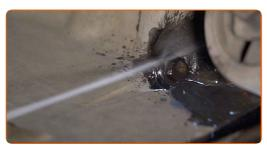
Unscrew the drain plug. Use a drive socket #24. Use a ratchet wrench.
