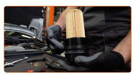
14.1 Install a new oil filter housing cover and tighten it.
