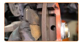
Replacement: brake pads – MERCEDES-BENZ W124 Coupe (C124). Tip from AUTODOC:
