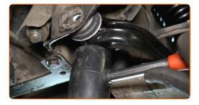
Install the fastening bolts. Use a rubber mallet.
