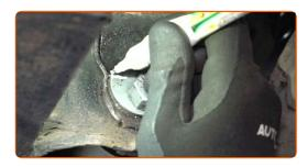
Unscrew the rear fastener of the control arm. Use a combination spanner #22. Use a drive socket #22. Use a ratchet wrench.
