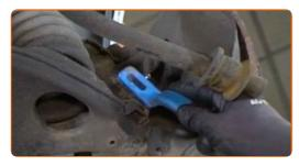
Attach the anti-roll bar to the suspension arms. Use a crowbar.
