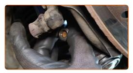
Tighten the fastener connecting the ball joint to the steering knuckle. Use a combination spanner #19. Use a drive socket #19. Use a torque wrench. Tighten it to 75 Nm torque.
