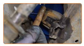
Disconnect the ball joint from the steering knuckle. Use a flat metal-working chisel. Use a hammer. Use a crowbar.
