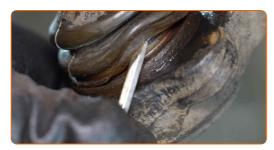
Dismantle the ball joint. Use a ball joint puller set.
