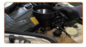
Pour coolant in the coolant reservoir.
