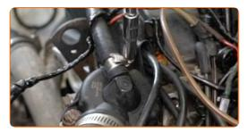
Detach the expansion tank hose from the thermostat housing.
