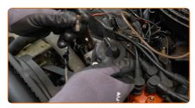
Remove the thermostat together with the housing.
