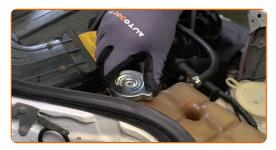
Screw on the coolant reservoir cap.
