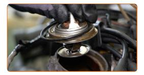
Replacement: engine thermostat – MERCEDES-BENZ W123 Coupe (C123).
