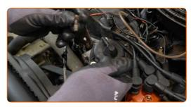
Remove the thermostat together with the housing.
