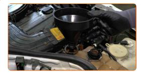
Pour coolant in the coolant reservoir.
