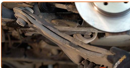
**17** Clean the mounting seats and the thread of the suspension arm. Use a wire brush. Use WD-40 spray.
