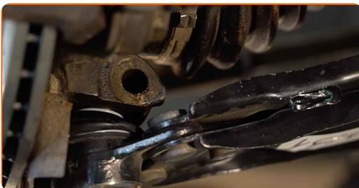
**22** Install the fastening bolt. Do not tighten it.
