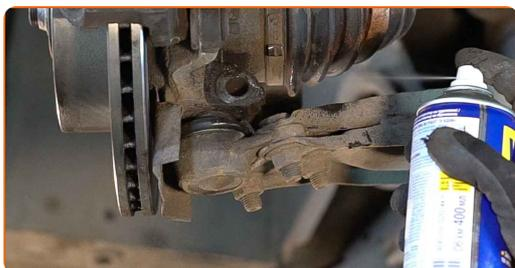
**14** Release the fastener connecting the ball joint to the steering knuckle. Use a flat metal-working chisel. Use a hammer.
