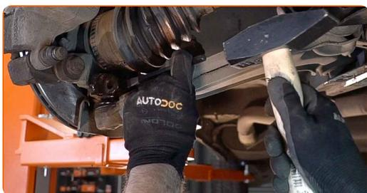
**15** Disconnect the spherical joint from the arm. Use a crowbar.
