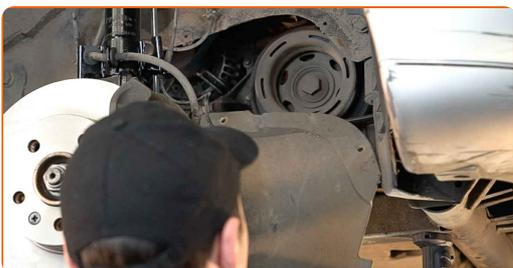
**10** Unscrew the front arm fastener. Use a combination spanner #18. Use a drive socket #19. Use a ratchet wrench.
