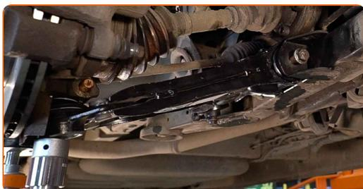
**25** Tighten the front fastener connecting the control arm to the subframe. Use a drive socket #19. Use a torque wrench. Tighten it to 155 nm torque.
