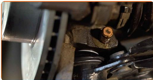
**23** Screw the rear arm fastener. Use a drive socket #19. Use a combination spanner #21. Use a ratchet wrench.
