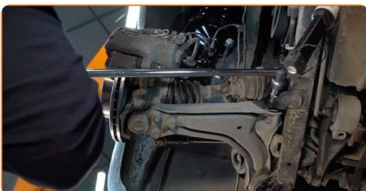
**11** Remove the fastening bolt. Use a crowbar.
