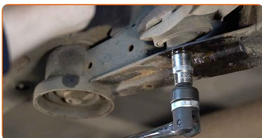
**13** Clean the fastener connecting the ball joint to the steering knuckle. Use WD-40 spray.
