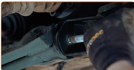
**12** Unscrew the rear arm fastener. Use a combination spanner #21. Use a drive socket #19. Use a ratchet wrench.
