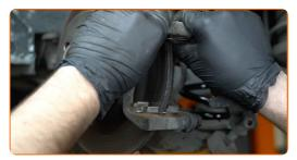
Remove the brake pad wear sensor from the brake pad. Use a flat screwdriver.
