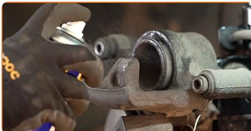
Replacement: brake discs – MERCEDES-BENZ VITO Box (W447). Tip:
