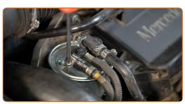
Disconnect the pipe from the fuel filter.
