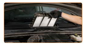
Install the cabin filter bracket. Use Torx T25. Use a torque wrench. Tighten it to 11 Nm torque.
