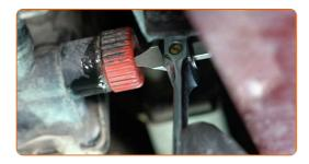
Clean the thermostat housing fasteners. Use a wire brush. Use all-purpose cleaning spray.
