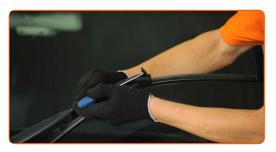
Remove the blade from the wiper arm.
