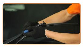
Remove the blade from the wiper arm.
