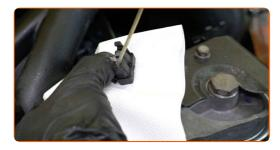
Plug in the connector of the coolant temperature sensor.
