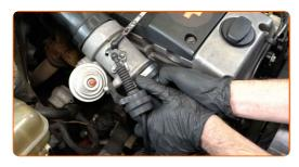
Tighten the air filter hose clamps. Use a drive socket #7. Use a ratchet wrench.
