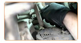
Loosen the coolant hose clamp. Use a drive socket #7. Use a ratchet wrench.
