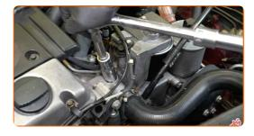
Install a new coolant temperature sensor.
