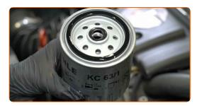
Clean the mounting seat of the fuel filter. Use all-purpose cleaning spray.
