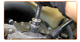
Loosen the fastening clamp of the fuel filter pipe. Use a Phillips screwdriver.
