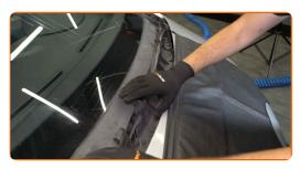
Screw in the fasteners of the lower part of the scuttle panel. Use a Phillips screwdriver.
