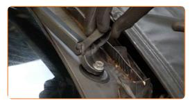
Clean the fasteners of the wiper arms. Use a wire brush. Use WD-40 spray.
