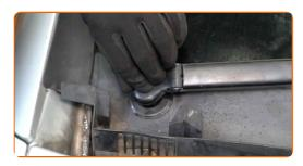
Install and secure the cowl grille. Use a Phillips screwdriver.
