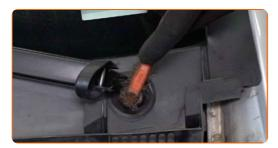
Unscrew the fasteners of the windscreen wiper arms. Use a drive socket #13. Use a ratchet wrench.
