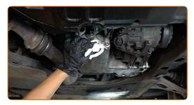
Screw in the new drainage plug and tighten it. Use a drive socket #18. Use a torque wrench. Tighten it to 29 Nm torque.
