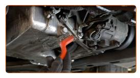
Unscrew the drain plug. Use a drive socket #18. Use a ratchet wrench.
