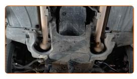
Tighten the fasteners of the oil pan lower cover. Use a drive socket #8. Use a ratchet wrench.
