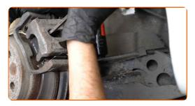
10 Remove the brake caliper.
