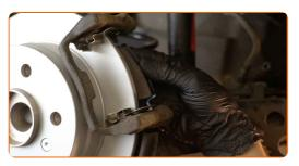
Replacement: brake pads – MERCEDES-BENZ VANEO (414). Tip from AUTODOC:
