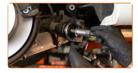
Install the brake caliper and fix it. Use a combination spanner #13. Use a combination spanner #15. Use a drive socket #13. Use a torque wrench. Tighten it to 35 Nm torque.
