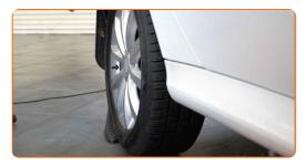
Loosen the wheel mounting bolts. Use wheel impact socket #H12.
