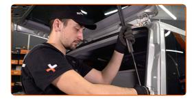
Install the new boot lid gas strut.
