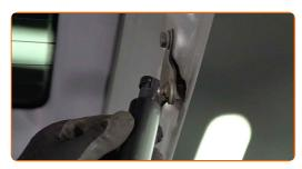
Snap on the circlip connecting the gas strut to the car body. Use a flat screwdriver.
