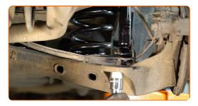
Tighten the lower fastener of the shock absorber. Use a drive socket #21. Use a torque wrench. Tighten it to 133 Nm torque.
