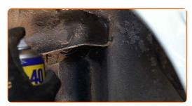
Unscrew the lower fastener of the shock absorber. Use a drive socket #21. Use a crowbar. Use a tap wrench.
