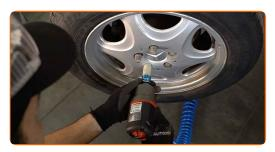
Lower the car and working in a cross order, tighten the wheel bolts. Use a torque wrench. Tighten it to 175 Nm torque.
