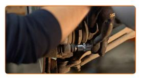
10 Remove the brake caliper.
