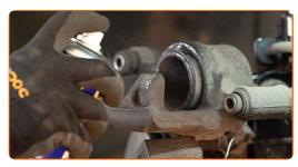
Press in the brake caliper piston. Use brake caliper wind back tool.
