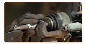
Treat the brake caliper bracket where it contacts the brake pads. Use anti-squeal paste.
