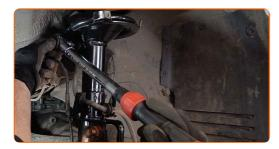
Tighten the fastener connecting the stabilizer link to the stabilizer bar. Use a drive socket #16. Use a combination spanner #16. Use a torque wrench. Tighten it to 62 Nm torque.
