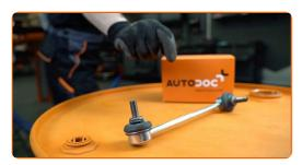
Tighten the fastener connecting the stabilizer link to the shock strut. Use a drive socket #16. Use a combination spanner #16. Use a torque wrench. Tighten it to 62 Nm torque.
