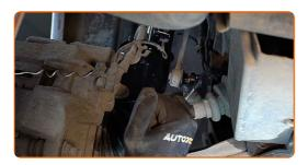
Unscrew the fastener connecting the stabilizer link to the shock strut. Use a combination spanner #16. Use a drive socket #16.
