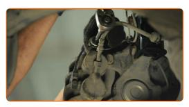
Connect the brake pad wear sensor plug.
