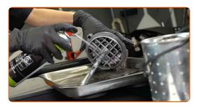
17 Install a new oil filter cap seal.
