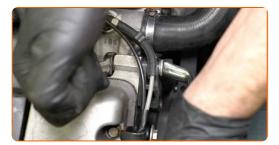
Use a lever of the correct diameter to loosen the tensioner and remove the fastening bolt. Use a 3/8" square drive extension bar.
