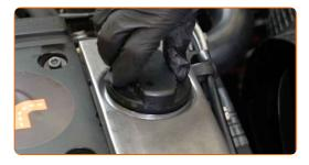
Tighten the oil filler cap.
