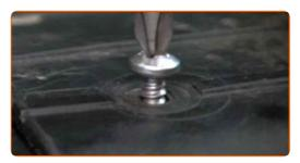
Screw in the inlet pipe fasteners. Use a Phillips screwdriver. Use a drive socket #10. Use a ratchet wrench.
