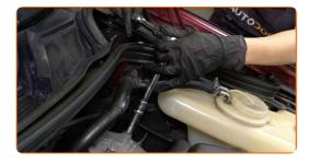
Remove the oil filter housing cap.
