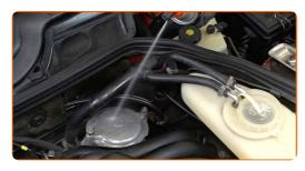
6 Unscrew the fasteners of the oil filter housing cap. Use a drive socket #13. Use a ratchet wrench.
