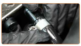
Replacement: fuel filter – MERCEDES-BENZ T1/TN Platform/Chassis.
