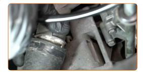
Replacement: temperature sensor and engine thermostat – MERCEDES-BENZ T1 Van (601, 611). AUTODOC recommends:
