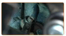
Drain the coolant from the engine.
