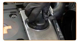
Tighten the oil filler cap.
