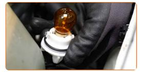
Install the turn signal light bulb holder by turning it approx. 30°.
