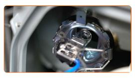
Detach the connector of the low and high beam bulb.
