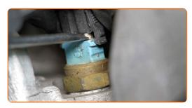
Clean the coolant temperature sensor. Use a wire brush. Use all-purpose cleaning spray.
