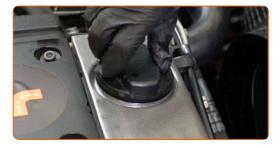
Tighten the oil filler cap.
