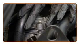
Tighten the fasteners of the oil filter housing cap. Use a drive socket #13. Use a torque wrench. Tighten it to 25 Nm torque.
