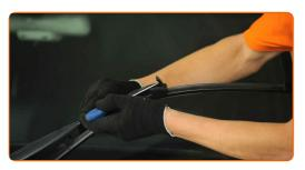
Remove the blade from the wiper arm.
