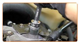
Loosen the fastening clamp of the fuel filter pipe. Use a Phillips screwdriver.
