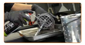
17 Install a new oil filter cap seal.
