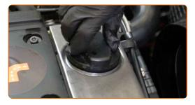
Tighten the oil filler cap.
